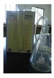
We have developed a unique procedure, which will measure the maturity of the compost. Maturity of the compost indicates whether it is ready for application to the field. This is the most important test for effluent based composting. It is easy to use this equipment. It takes only 3 hours to conduct each trial.
